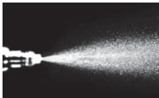
Injector spray pattern after P.i. treatment.
